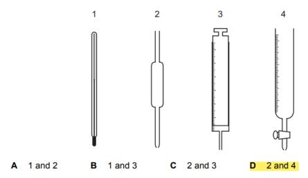
A thermometer and gas syringe are not used in titration.
