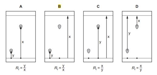
$R_f = rac{ ext{Distance travelled by substance}}{ ext{Distance travelled by solvent}}$
